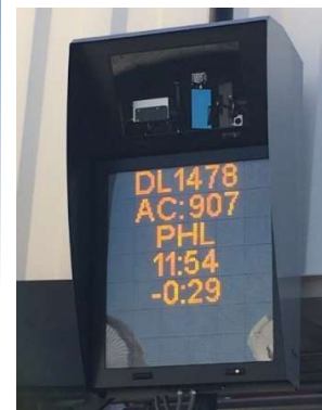
AVDGS T1 Ramp display unit
