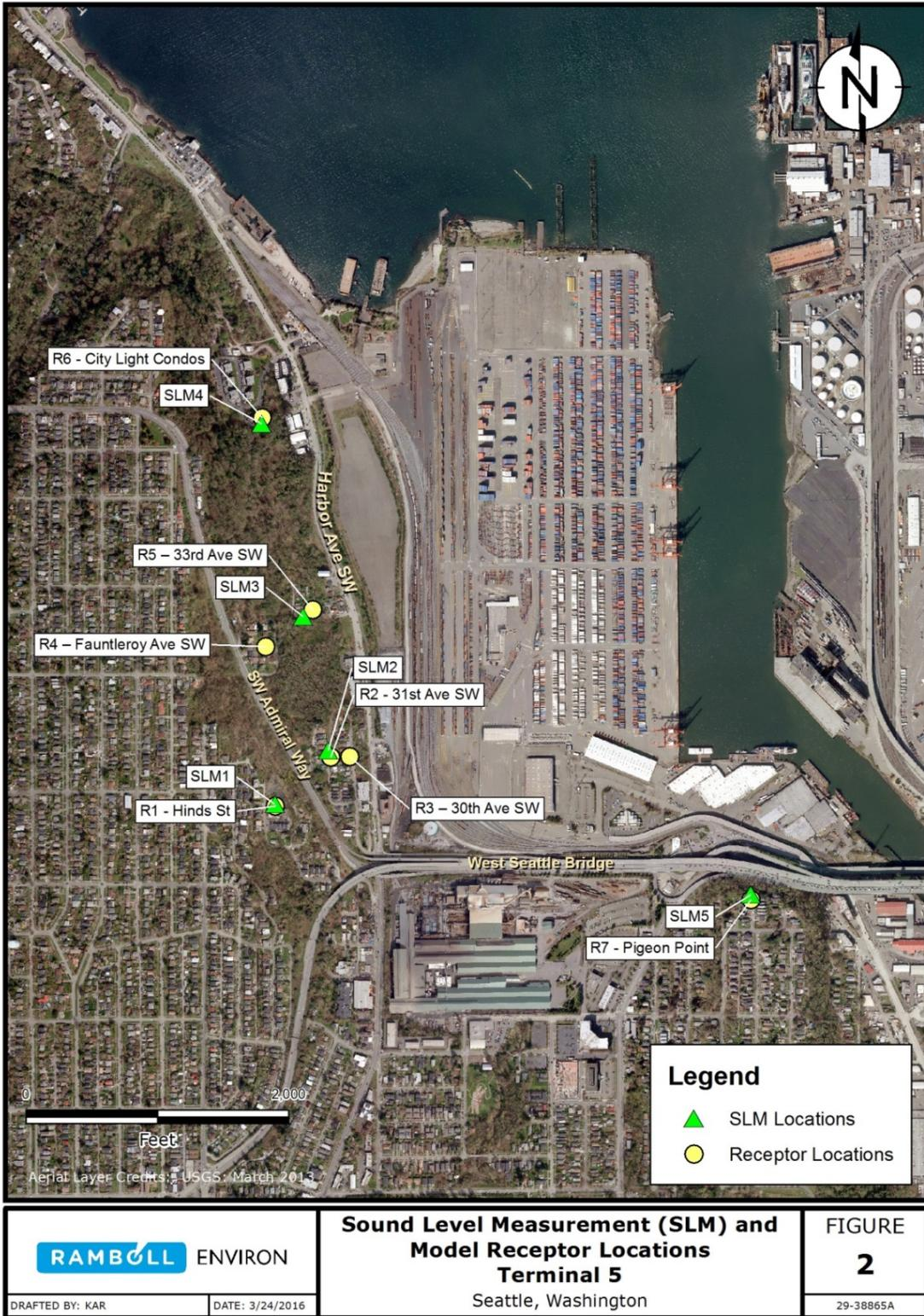
Figure 3.6.2: Sound Level Measurement (SLM) and Model Receptor Locations
