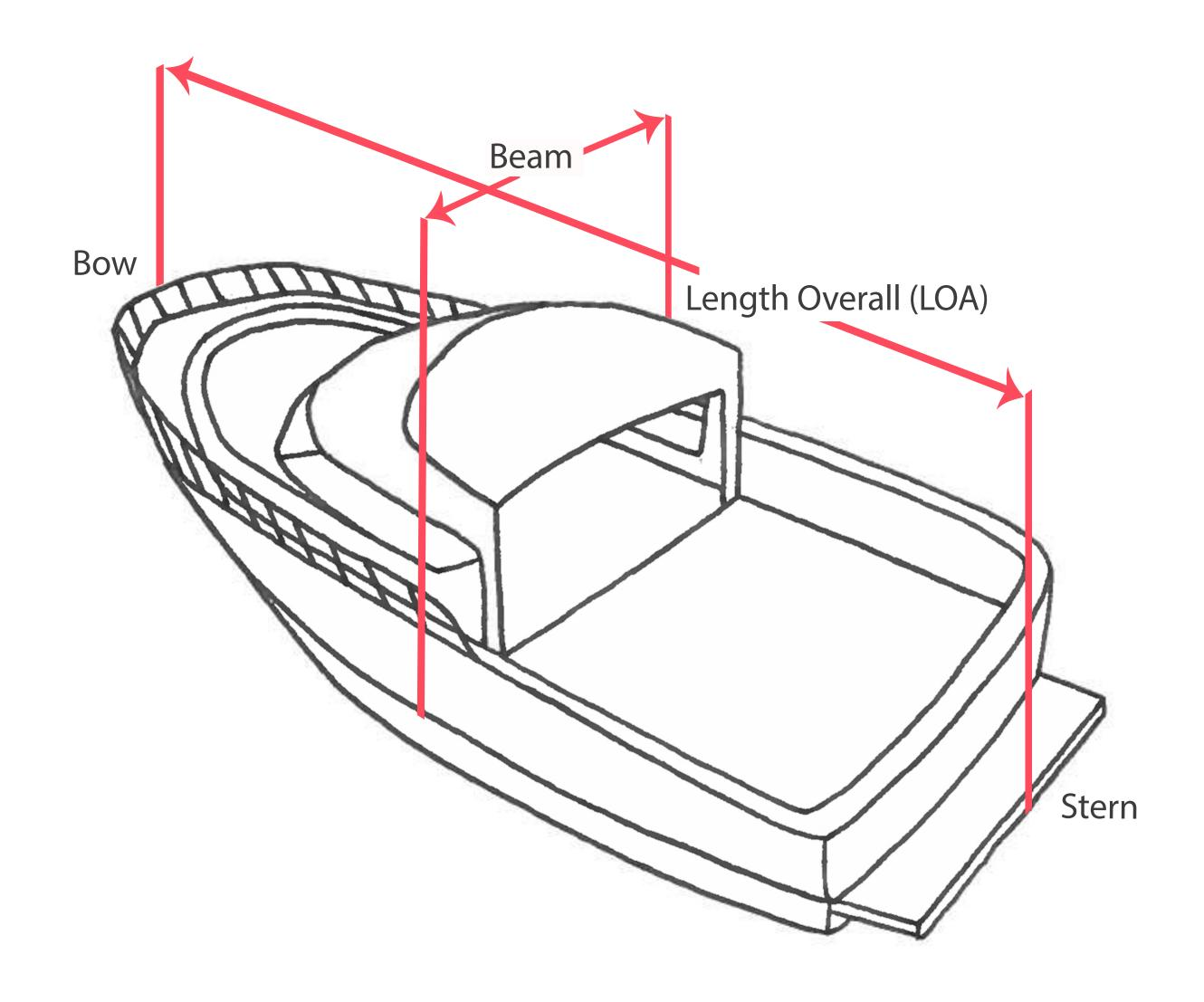
Length overall (LOA) must include any rear deck extensions or swim platforms on the stern to the forwardmost fixed appendage of the bow or bow pulpit
