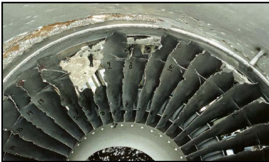
This engine on a Boeing-737 sustained major damage when a female eider duck was ingested during landing at an airport in Maine, November 1995.
