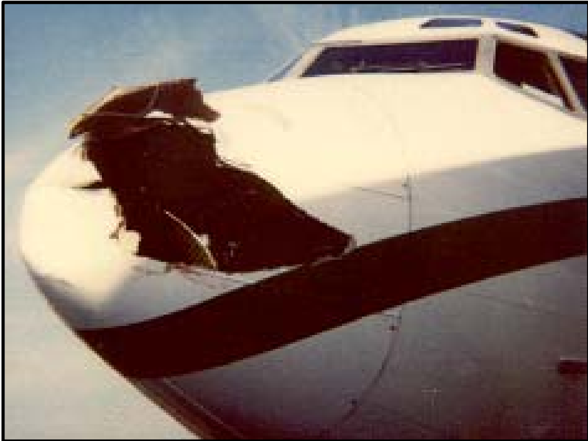
On September 27, 1990 this Boeing 727 struck a common loon on departure from SEA.
