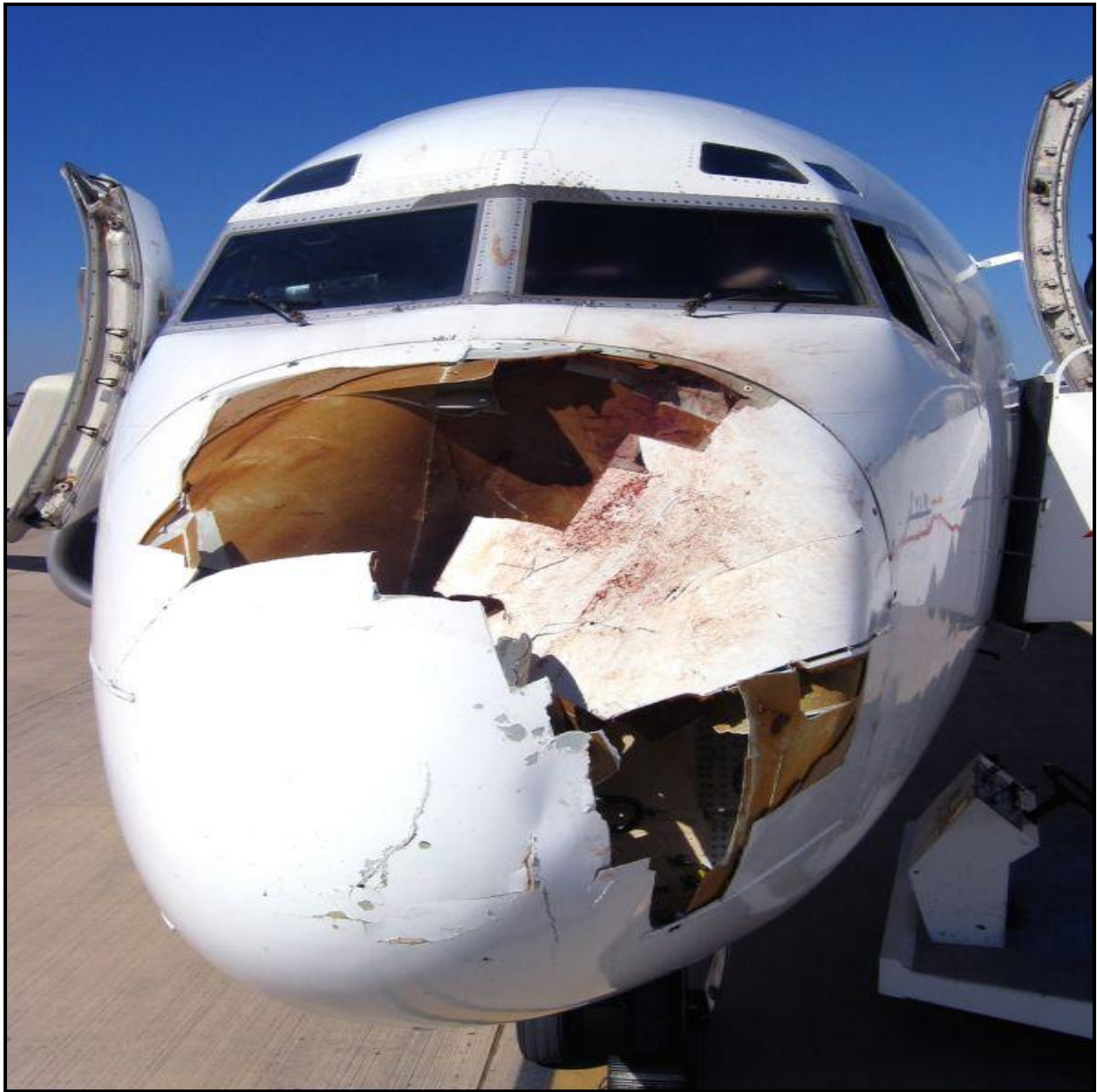
Damage resulting from a high speed strike with a single gull.
