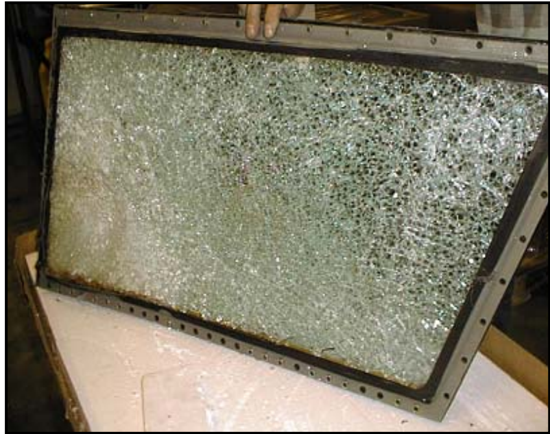
A 737-400 aircraft, flying at 10,000' and 314 knots, sustained significant windscreen damage when colliding with a snow goose. The higher speeds common at these altitude result in the greater likelihood of more severe damage.
