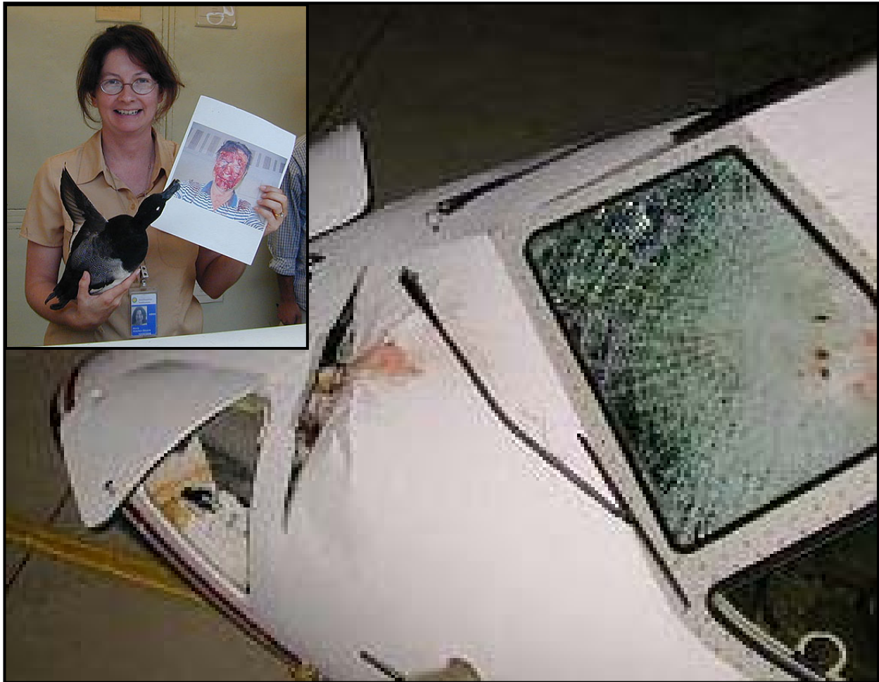
Waterfowl, such as these scaup, have been identified to species by the Smithsonian Institution and are known to cause great damage and personal injury as seen here. Several hrs after departing SEA for Medford, OR, the pilot was injured after his Dash 8 aircraft struck a flock of scaup.
