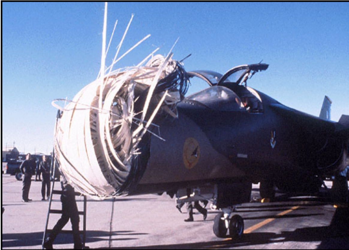
The composite raydome was destroyed after this F-111 collided with a Red-tailed Hawk Cannon AFB, New Mexico (Photo courtesy USAF).
