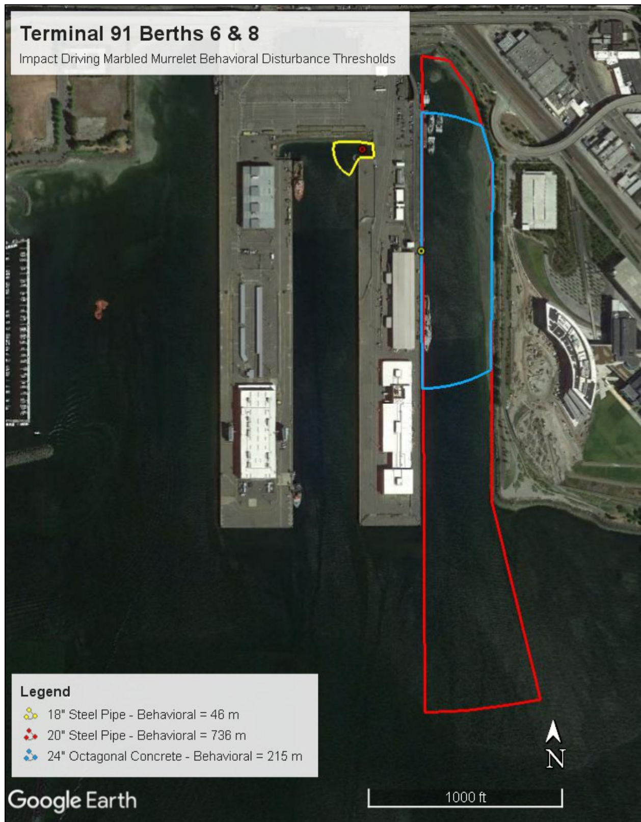
Figure 7. Distances to marbled murrelet behavioral disturbance thresholds for impact pile driving 18" (guide pile for relocated small boat storage) and 20" steel pipe pile and 24" octagonal concrete pile.
