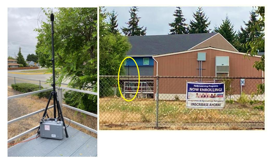
Portable noise monitoring microphone mast and equipment box was placed on the metal deck on the south side of the school's portable classrooms P-3 and P-4. From the main street, 14<sup>th</sup> Ave SW the mast and equipment is barely visible. Note black microphone mast in yellow photo above.
