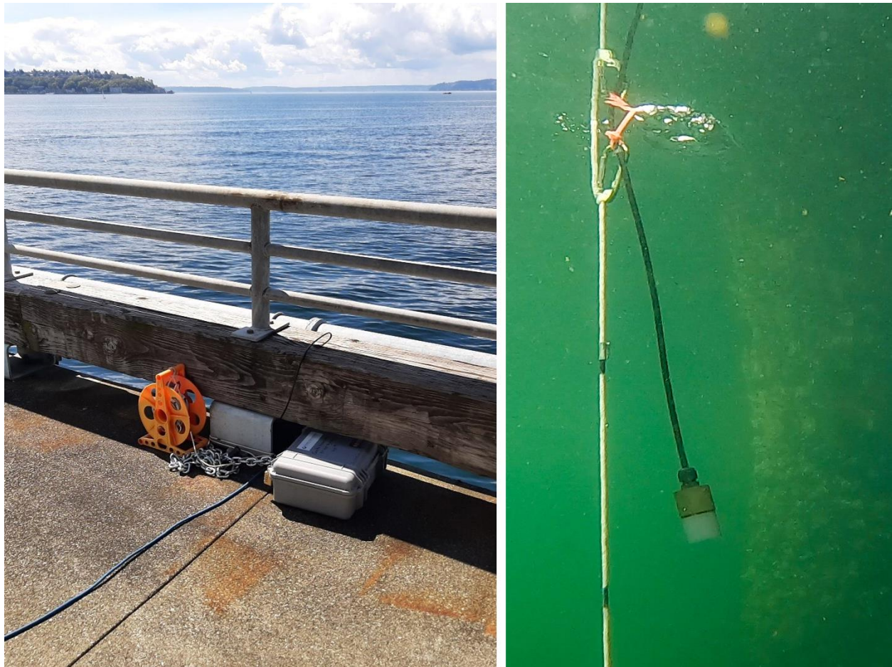
Figure 16. Equipment recording ambient underwater noise in Elliott Bay. Credit: Sasha Ertl/Grette Associates and Port of Seattle
