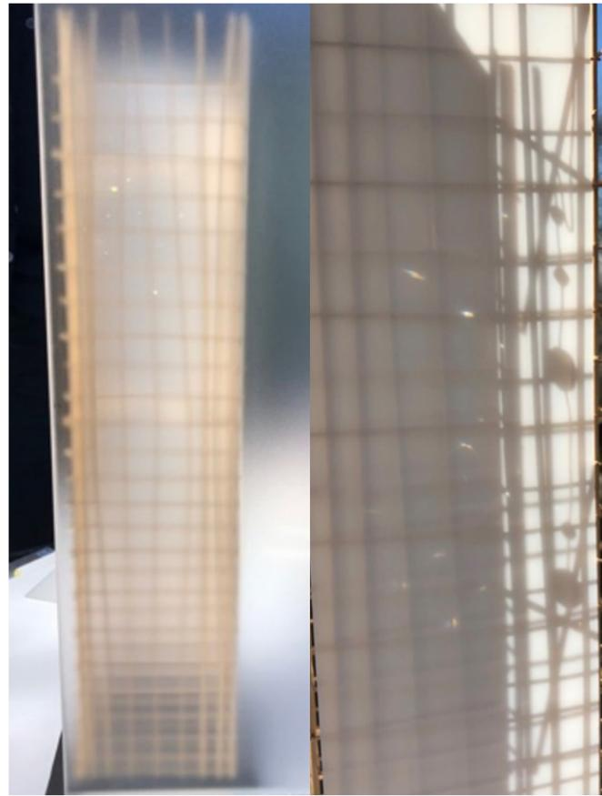
Model of existing tower structure with light-diffusing cladding on front and prisms hanging behind.
