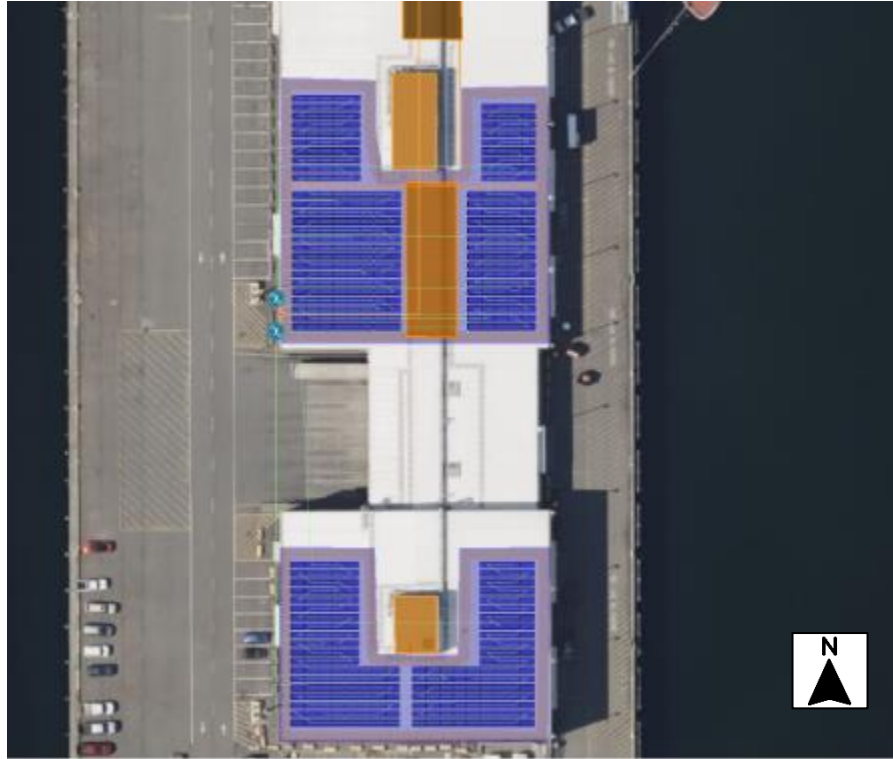
Figure 31: Helioscope Model for Terminal 91 C-175 showing keepouts (orange) and other model details. Keepout areas typically include mechanical equipment, access pathways, skylights, and roof drains.
