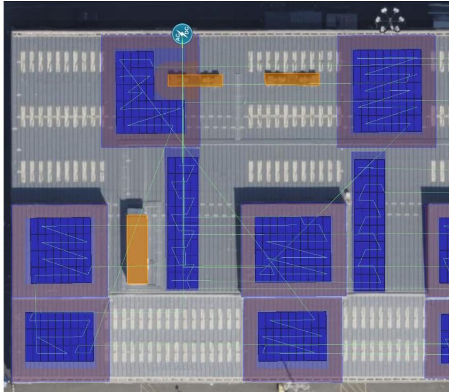
Figure 3: T91 A-1 Warehouse Building with “keepouts” in orange to provide more accurate shading in modeling. Heights and dimensions are then confirmed through site walks for shortlist facilities.
