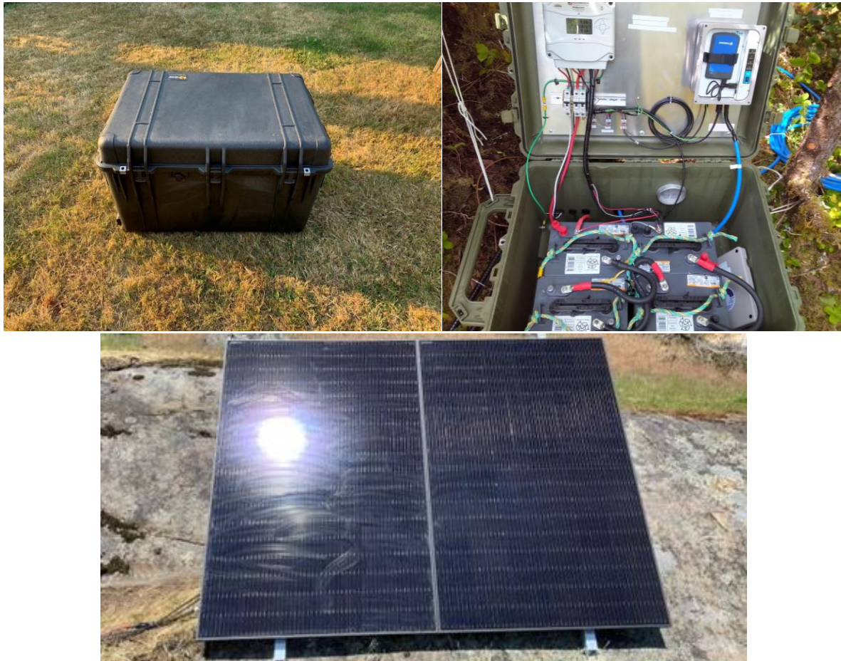
Figure 2: Sample of the shore station box and solar panel (if required)
