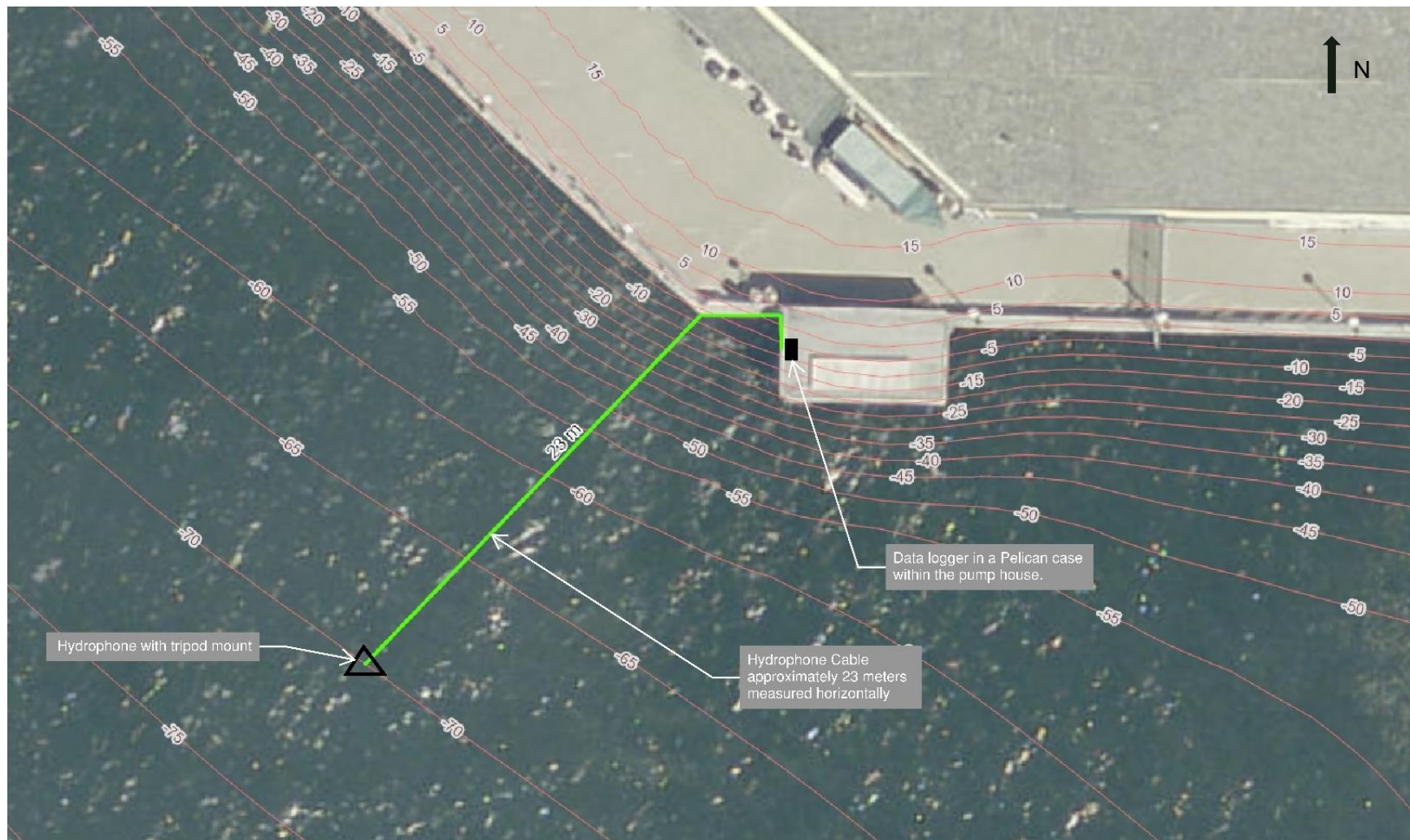
Figure 12: Seattle Aquarium Pier – Hydrophone Equipment Schematic
